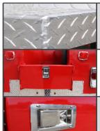
Rugged, corrosion-resistant 5052-H32 grade aluminum body. Remarkably, the 56 CA model wighs less than 725 lbs. (40 CA also available)
